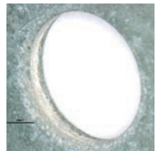
16 months 10% red rust 70% white rust
