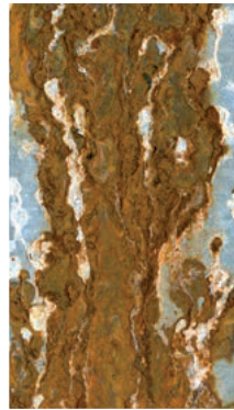
Hot dip galvanised 20 µm after 6 weeks
